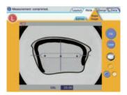
The optional partial step package provides automatic measurement of the partial step data of the demo lens. With partial step edging of the Multifunction Edger Me 1200\*, the partial step package allows the prescribed spectacle lenses to be mounted into the frame of sports sunglasses, and helps to meet the request of a demanding customer. \* Available for PLB-8S and PLB-2R8S types
